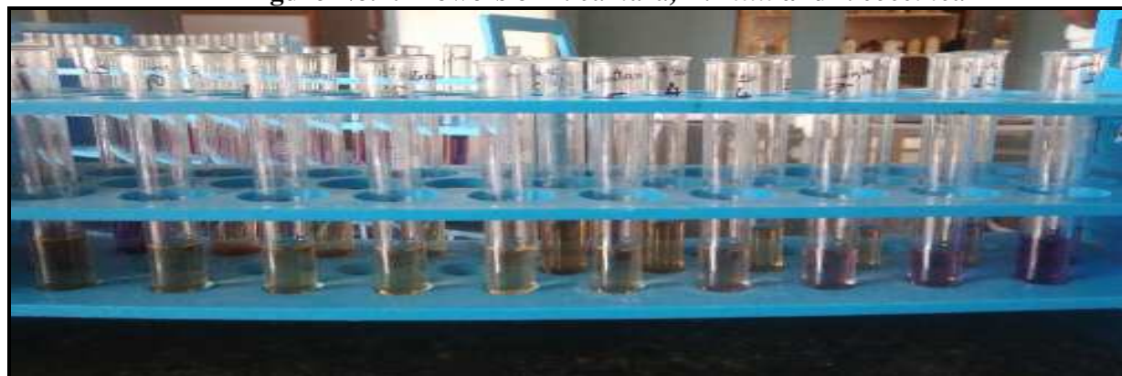
Figure No.2: Test tubes showing the inhibition of free radicals
